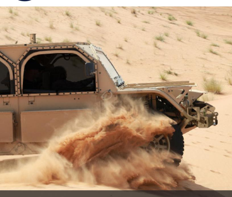
The Flyer® 72 is a non-developmental item, purpose-built, lightweight vehicle designed to meet complex mission sets. Selected by the U.S. Special Operations Command (USSOCOM) as the vehicle of choice for their Ground Mobility 1.1 (GMV 1.1) program, at 72" wide it is capable of internal transport in the CH-47 and C-130 aircraft.
